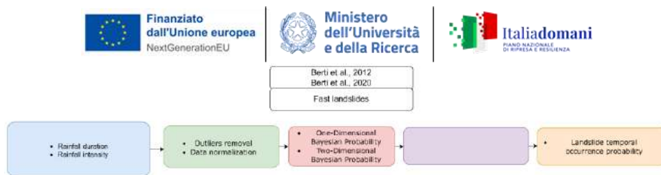
Figure 7 – Toolchain for landslide temporal occurrence probability (Berti et al., 2012, 2020)
