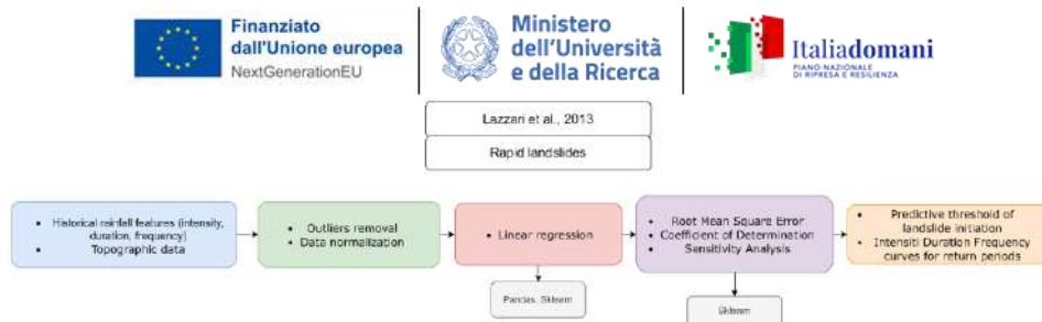
Figure 5 – Toolchain for intensity duration frequency curves (Lazzari et al., 2013)
