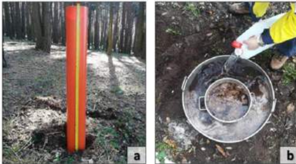
Figure 13. Single (a) and double (b) ring infiltrometers used to perform falling head infiltration tests in Sorico.
