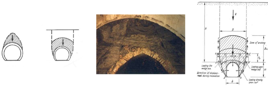
Figure 26: Picture that highlights the position and size of the dead load volume as observed during the enlargement of a railway tunnel and scheme of the Terzaghi load model as reported by Szechy (1970)
