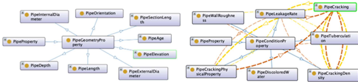
Figure 6: Fragments of semantic models of the pipe property entity adopted from ATU ontology: (left) the pipe geometry property hierarchy; (right) the pipe conditions and their links.
