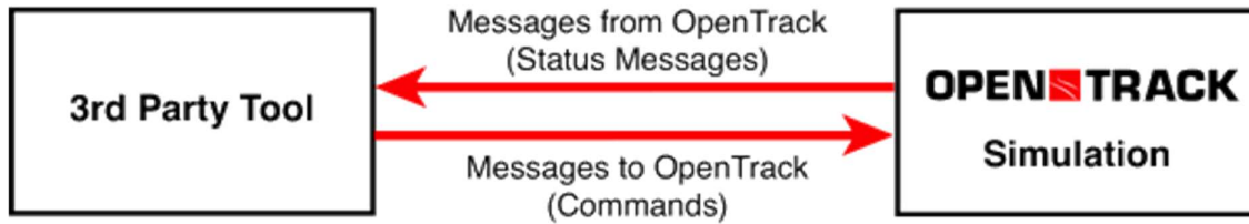
Figure 1: Interfacing mechanism with OpenTrack
