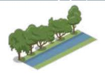
**Bioretention areas**: Bioretention areas, including rain gardens and bioswales, are vegetated trenches designed to capture stormwater runoff at specific locations, helping to manage rainwater effectively.
