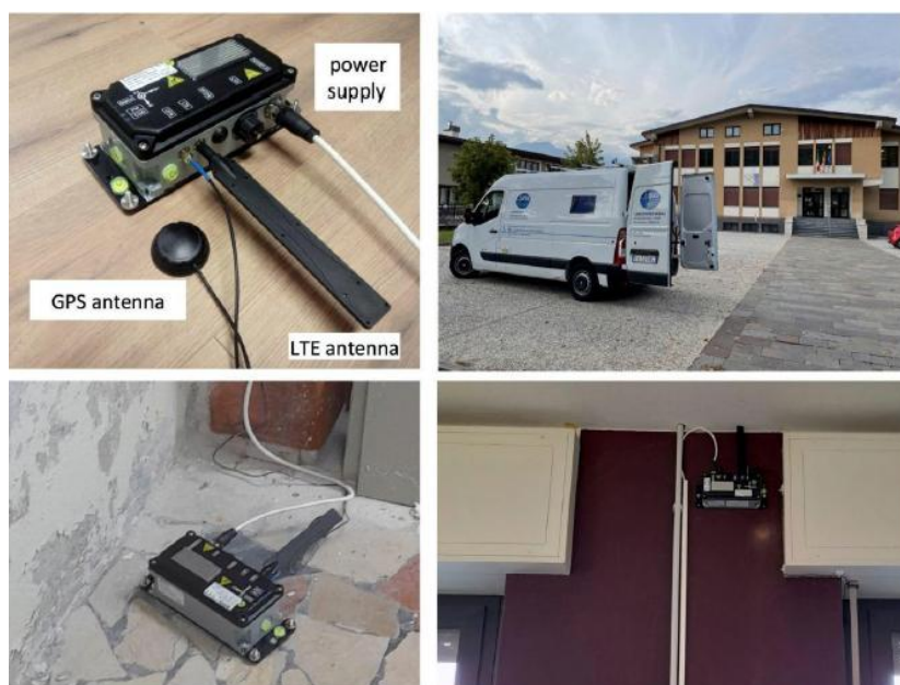
Figure 2 Accelerometers installed at the top and at the bottom of a public building.
