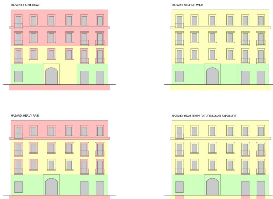
Figure 18. Example of maps to identify the areas of a façade that have the greatest impact on the surroundings if a potentially disruptive event happens, such as an earthquake, heavy rainfall, high temperature, or windstorm.
