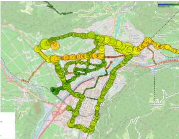
Figure 51. Mobile temperature data from MeteoTrackers: Full month of April example of over one bus. The size of circle represents the amount of data collected whereas the color bar represents the average temperature.
