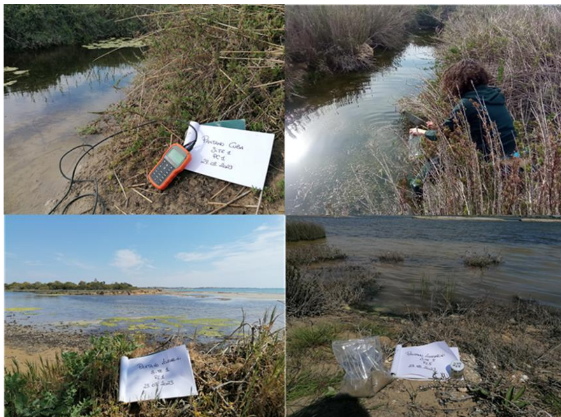
Figure 7. Sediment sampling surveys at the lagoons. Each sampling station is identified by its site name and acronym, with coordinates and the date of the survey also noted. Three sediment samples were collected from each site for grain-size, micro-, and macrobenthic analyses.
