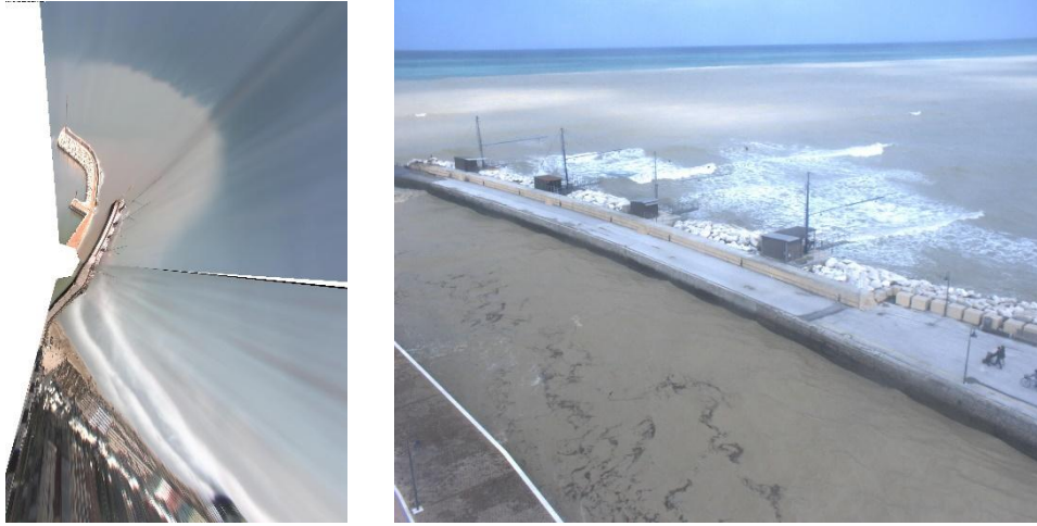
Figure 14. Left: SGS time-exposure image showing a plume caused by the combination of river discharge and NNE waves. Right: video frame acquired by one of the SGS cameras, showing debris on the water surface that were detected by the PTV algorithm.
