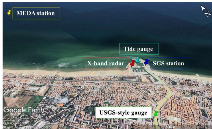
Figure 7. Instrumentation installed within and nearby the MRE.
