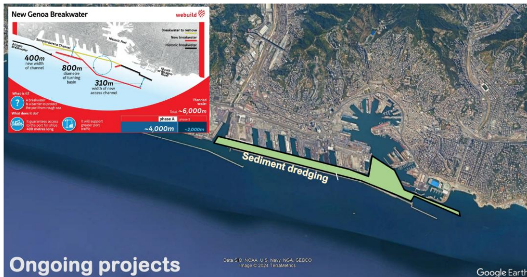
Figure 7b. Sketch of the new Genoa Breakwater: the green area represents the basin to be dredged.
