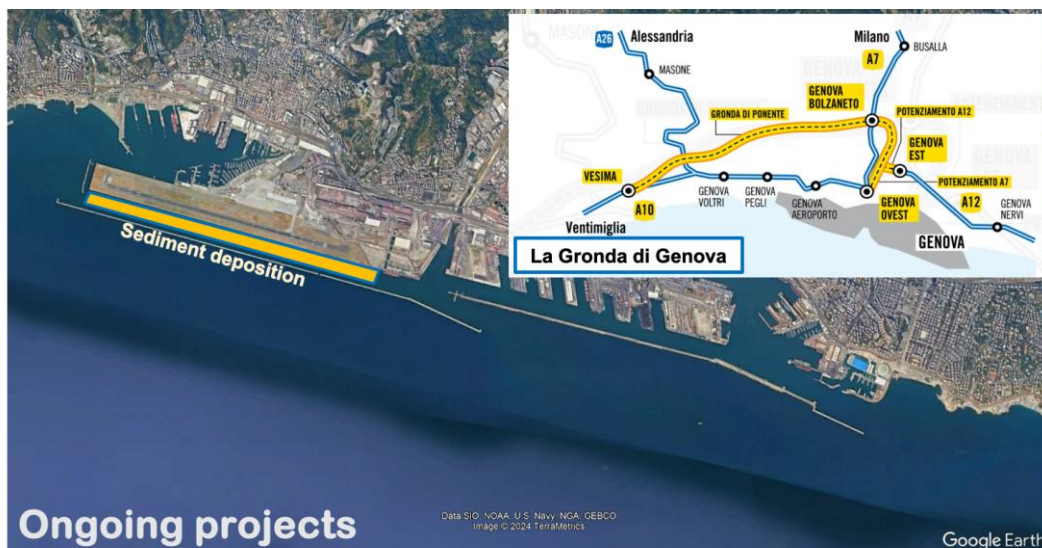
Figure 8. Sediments dredged from basin 7b, and the debris issued from the slurry duct will be dumped in the yellow area to enlarge the airport.
