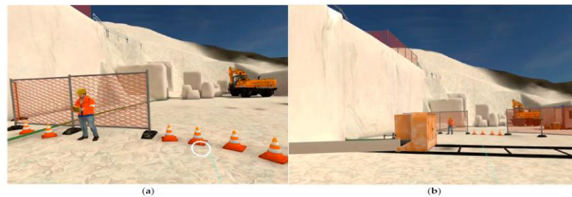
Figure 7. VR course on primary cutting upstream (SO1). Before starting horizontal cutting, the user interacts with the pointer, verifies the compliance of the operational phase checking the safety distances from the machine (a), positioning the diamond wire guards in order to avoid whiplash in the event of wire breakage during horizontal cutting (b). Source: authors' processing by Software Simulation version 1.2.1.
