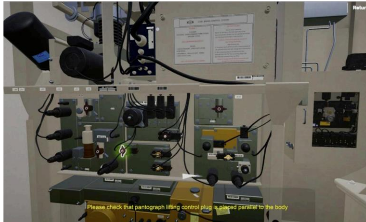
Figure 19: VR instructions on how to handle the most common faults in a locomotive for crew training. Reproduced from [35], © 2023 The Author(s), distributed under the Creative Commons Attribution License (CC BY 4.0).
