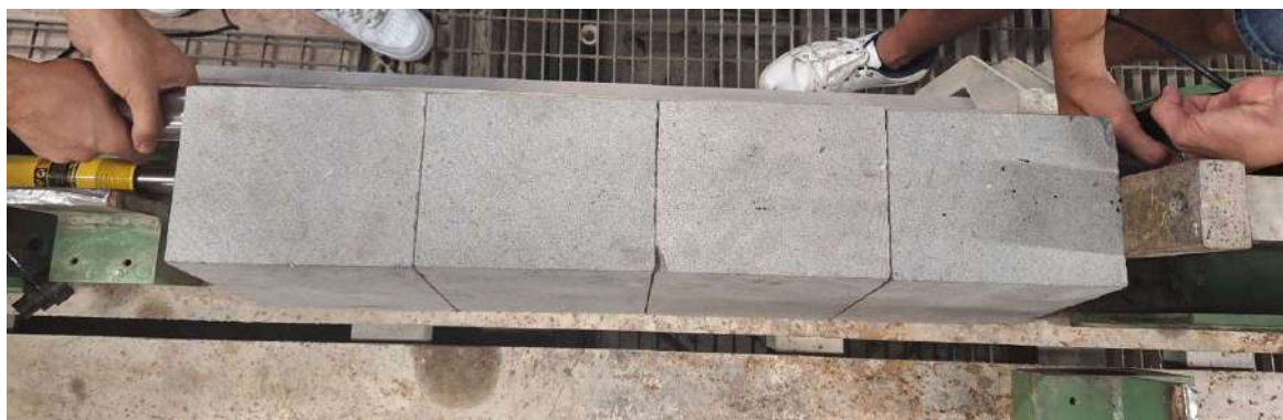
Figure 147. Ultrasonic tests using a laboratory setup compound by four basalt blocks by applying different pressures.
