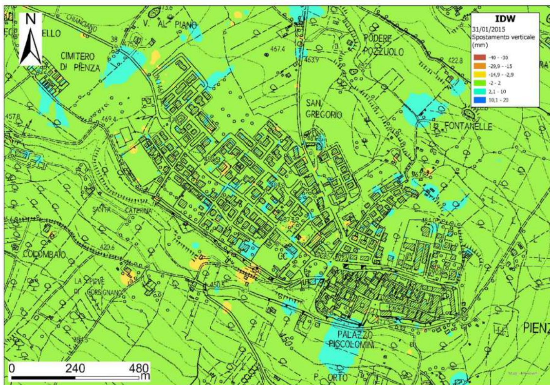
Figure 79. Interpolation of CSK synthetic PS data showing vertical displacement as of January 31, 2015, based on CTR 10k for the Region of Tuscany
