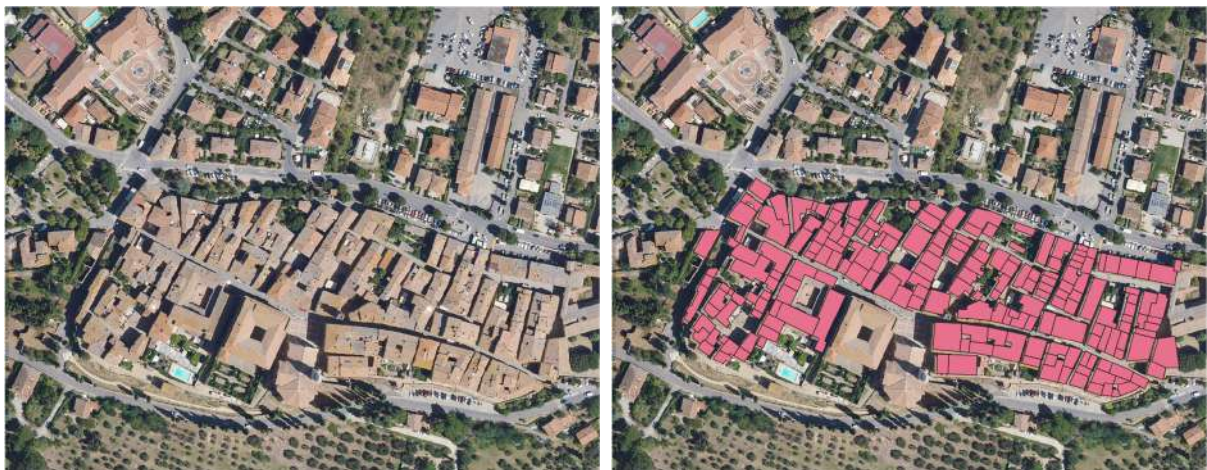
Figure 57. a) aerial view of the historical center of Pienza; b) realization of the geometrical shapes for each SU considered in the research.
