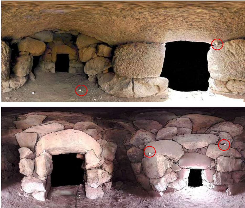
Figure 110. 360-degree views from the TLS, showing the arrangement of the polystyrene spheres.
