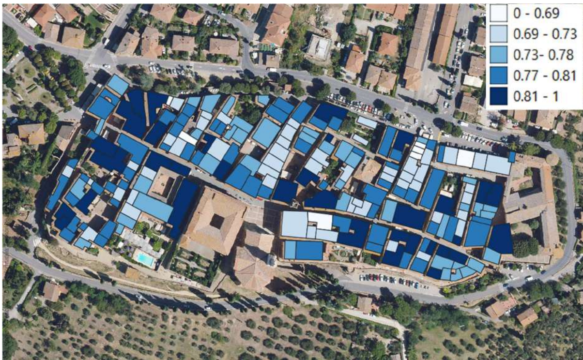
Figure 71. Seismic vulnerability indexes obtained for the different structural units of the historical centre.
