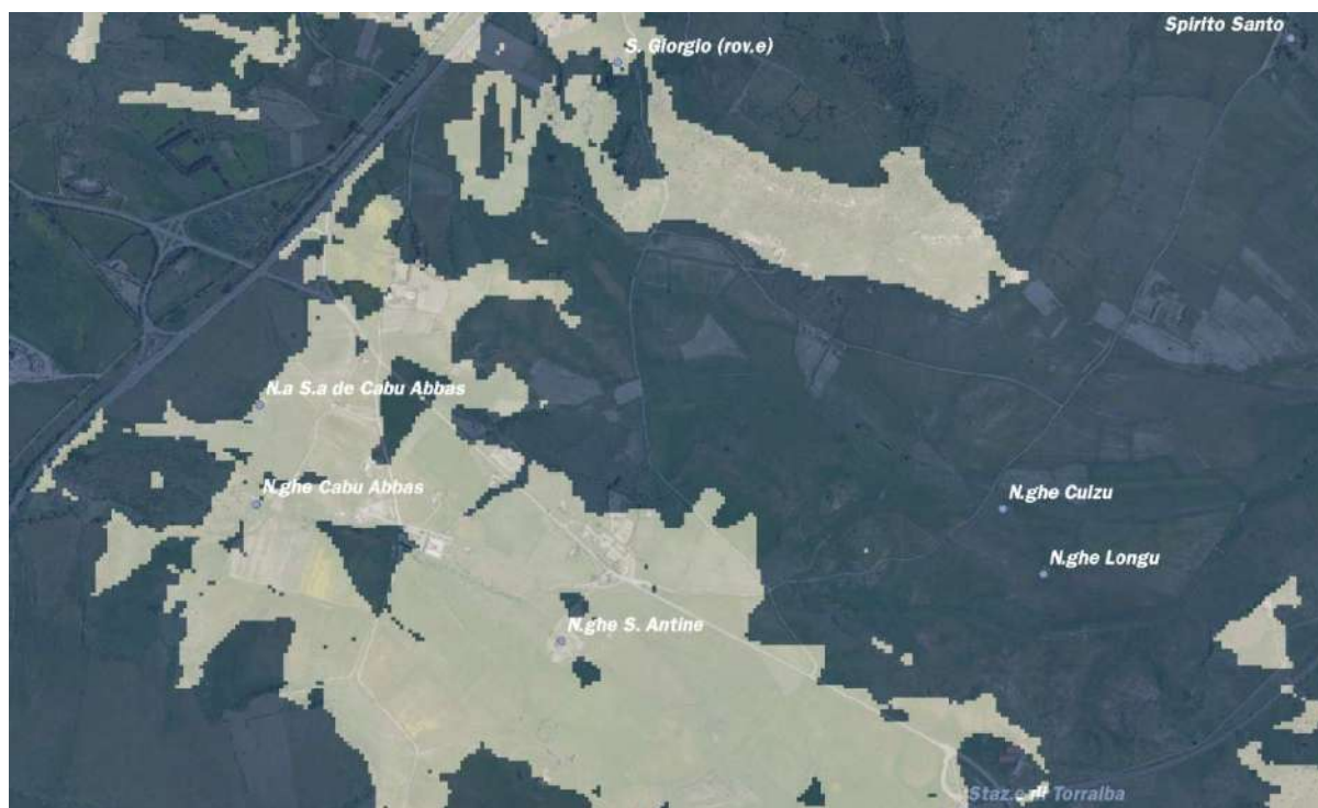
Figure 213. Simulation of visual cones with a viewpoint set at human height (1.60 m) near the Nuraghe Santu Antine. The obstructed portion of the view is shown in dark.
