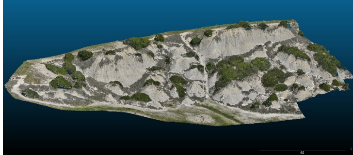
Figure 2: 3D model of study area derived from SfM
