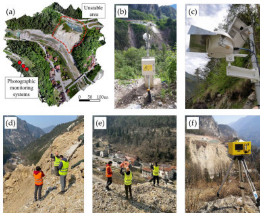
Figure 2: (a) Aerial view of the landslide with camera locations; (b,c) view of one of the monitoring systems; GPS surveys of (d) a corner and (e) a reference sphere, both located on the big scarp edge of the slope; and (f) laser scanning survey of the landslide.
