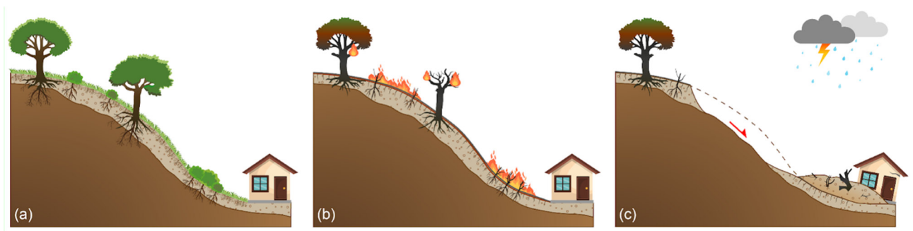
Figure 6.6: Evolution of a slope affected first by wildfire and subsequently by rainfall, leading to instability. (a) Pre-fire condition: slope covered by soil and vegetation. (b) Wildfire event with varying burn severity, causing alterations in soil and vegetation. (c) Post-fire rainfall triggering a shallow landslide, with consequent damage to the built environment.
