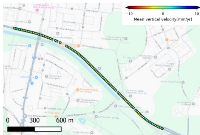
Figure 7-4 – Example of merged InSAR data for a specific bridge near Mantova: mean vertical velocity computed for the 2015-2021 time window.
