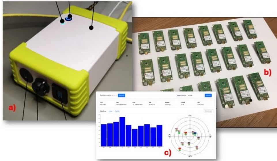
Figure 5. a) the first LZERO prototype developed by OGS and used as the first sample to produce more pieces. b) The LZERO Core Card (LLC) an electronic board developed by OGS mounting the U-BLOX ZED F9P GNSS chip receiver and included in the LZERO NET device. c) part of the interface which is under development for LZERO NET.
