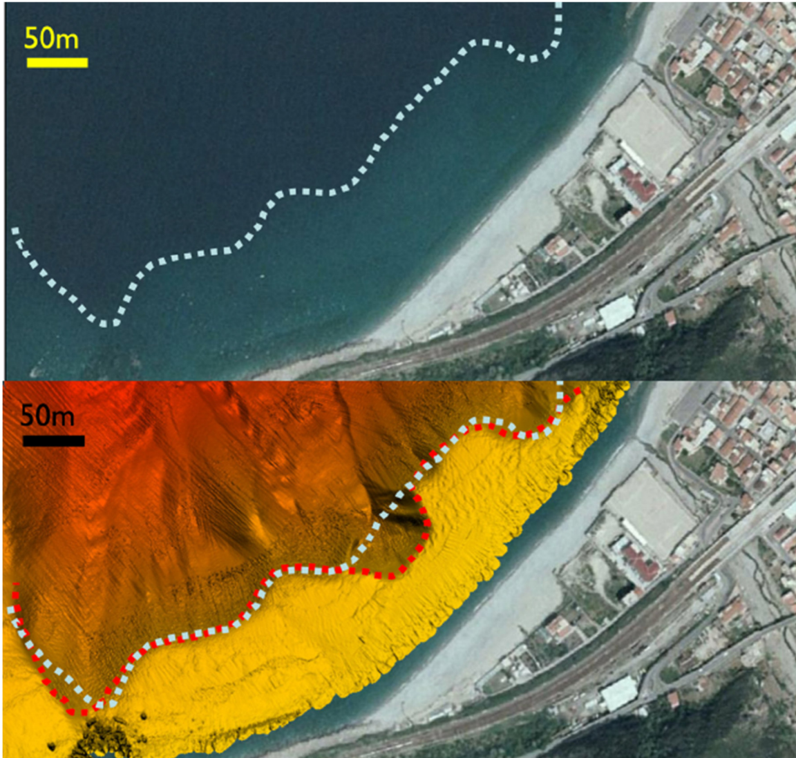
Figure 22. In the upper image the color change is produced by a sharp slope break with a sudden depth increase (similar to Figure 21). In the central image the difference in color has been mapped by a dashed white line. In the lower image multibeam echosounder data defines the morphobathymetry of the area, where active erosion is going on, as witnessed by the arcuate bedforms at the center of the channels. The red dashed line defines the slope break. The difference between the two lines highlights the occurrence of a small submarine landslide between the two surveys. Note the short distance from the coast (up to less than 100m) and the presence of houses, main roads and railroad threatened by coastal erosion and eventually by tsunamis produced by large submarine landslides. Instead, the small landslide highlighted by the comparison between the two surveys was un-noticed. Problems due to coastline erosion is witnessed by artificial blocks emplaced at the shoreline in the lower left corner of the image, where the canyon head is closer to the shore.
