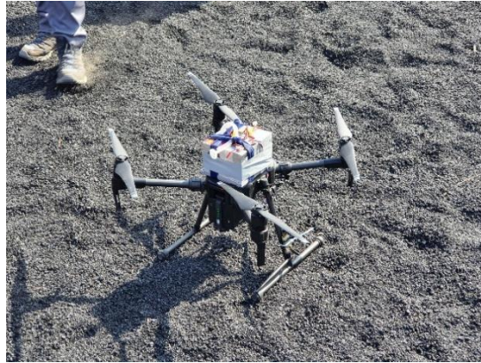
Figure 4.1.5: The drone and the transmission system
