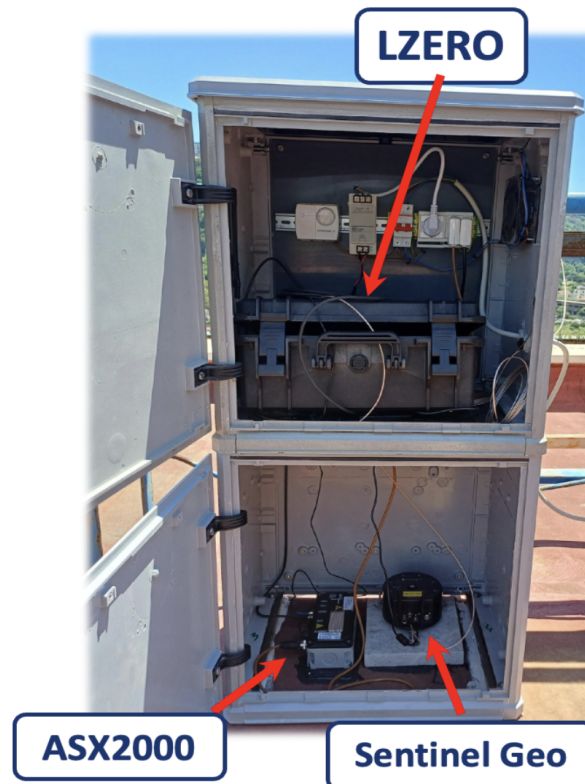
Figure 6. Installation of the multi-sensor monitoring system at the Piazzale Tecchio site (UNINA, Campi Flegrei area). Photographs document representative mounting configurations of the accelerometric (ADEL ASX2000), velocimetric (Lunitek Sentinel GEO) and GNSS (LZERO) sensors.
