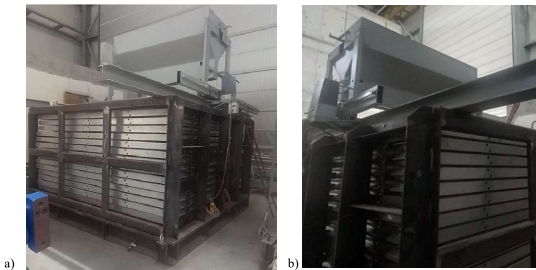
Figure 4: Pluviation system attached to a supporting frame above the laminar box at L.E.D.A.
