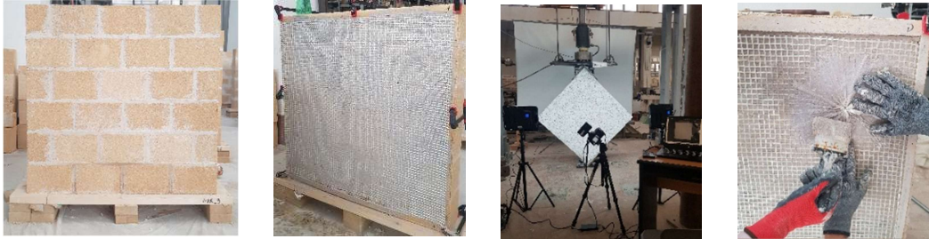
Figure 11: Masonry panels geometry, FRCM applications and test set-up.
