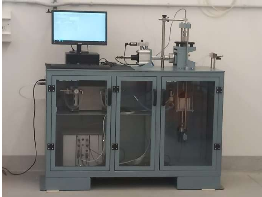
Figure 5: CDSS apparatus at the Soil Dynamics and Geotechnical Engineering Laboratory.
