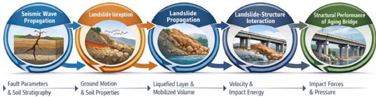
Figure 10: Schematic representation of the developed physics-based cascading multi-risk methodology for seismic assessment of aging bridge under seismic induced landslides. It is structured into five sequential computational modules (“rings”), each representing a distinct physical process and exchanging physically meaningful state variables.
