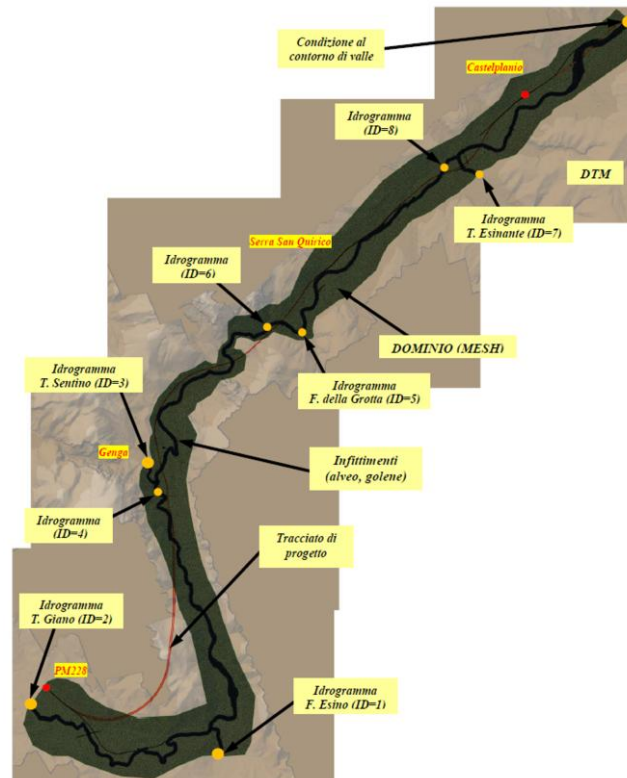
Figure 6.5 The two-dimensional numerical model of the Esino River.
