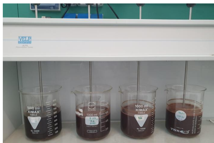
Figure 25: Jar test apparatus used for the batch tests
