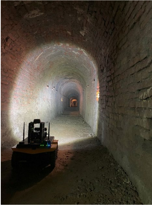
Figure 1 The ClearPath Jackal UGV rover equipped with sensors and lights navigating the underground tunnel system of Pietro Micca Civic Museum in Turin
