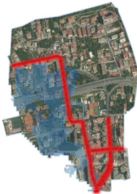
Figure 21 - Scenario ante: Inundation Map with over 2500 m3 of flooded volume.
